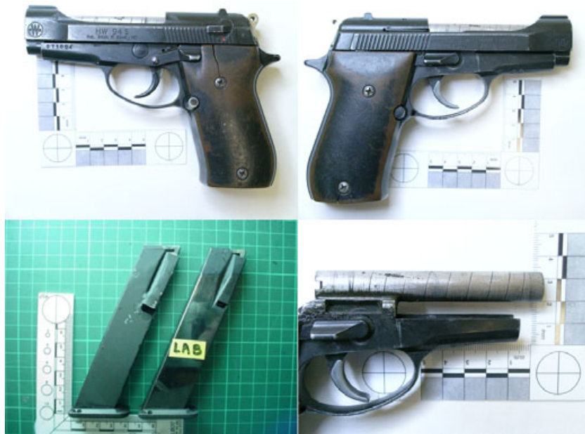
FIG. 5—Converted HW94S blank cartridge firing pistol (top row). Bottom left—showing a compatible modified magazine on the left and the unmodified BBM Bruni 92 magazine on the right. Bottom right—showing the replacement barrel.
