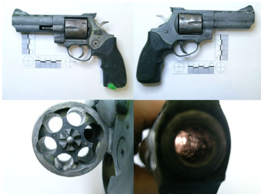
FIG. 9—Most common version of the converted self-contained gas cartridge revolver, aka “Brocock” (top row). Bottom left—chamber restrictions are removed. Bottom right—original rifled barrel sleeve removed. In this condition, the revolver is capable of firing conventional .38 Special caliber cartridges.
