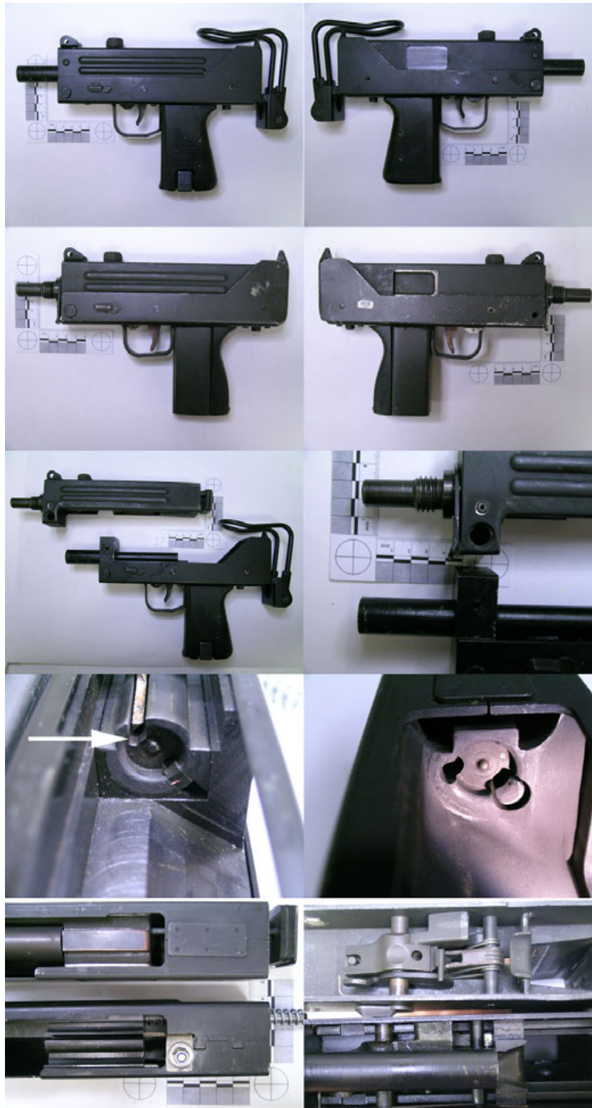
FIG. 7—Converted MAC-10 blank cartridge firing sub-machine gun (top row). Second row—original MAC-10 sub-machine gun. Third row left—barrel attached to upper receiver on original (top) and barrel attached to the lower receiver in blank firing version (bottom). Third row right—threaded muzzle on original (top), not present on blank firing copy (bottom). Fourth row left—breech face of blank firing version showing “lozenge” shaped ejector cut-out, marked with white arrow. Fourth row right—breech face of original, showing semi-circular shaped ejector cut-out. Bottom row left—ejector holding plate on underside of bolt on the blank firing version (bottom). Bottom row right—barrel covering the internal trigger mechanism on the blank firing version (bottom).
