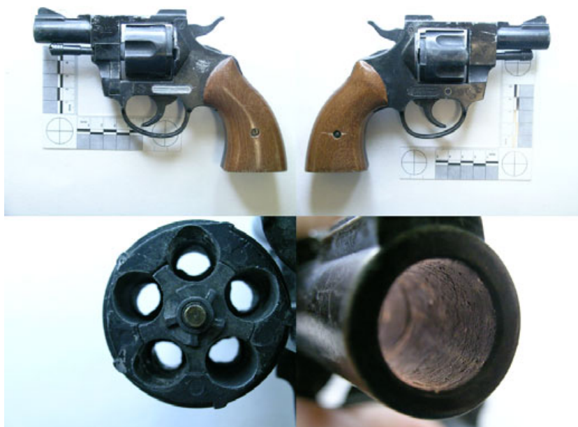
FIG. 8—Converted BBM Olympic 38 blank cartridge firing revolver (top row). Bottom left—partial chamber obstructions are removed. Bottom right—barrel obstruction is removed.
