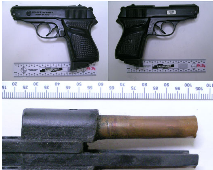
FIG. 3—Converted BBM Police blank cartridge firing pistol (top row). Bottom photograph showing the replacement barrel, which in this example is a piece of copper tubing.
