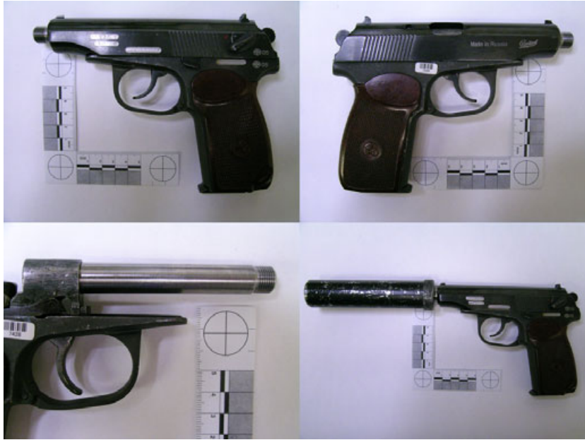
FIG. 6—Converted Baikal IZH-79 pistol (top row). Middle left—replacement barrel with threaded muzzle. Middle right—pistol fitted with sound moderator.
